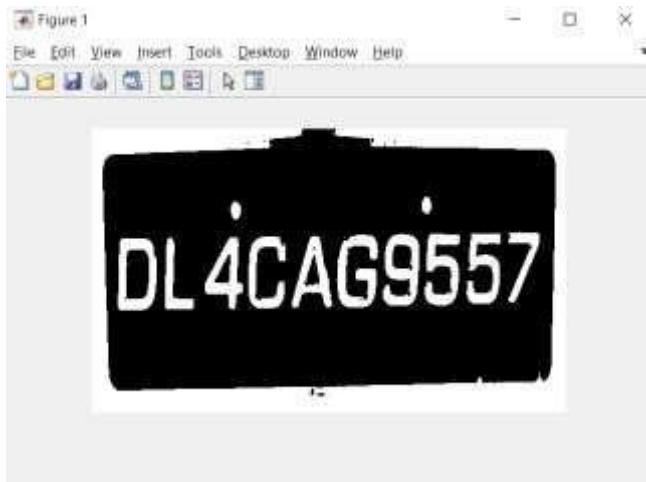
Fig. 2. RGB to B/W converted Image
