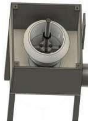
Figure 5: - Housing and coupling done inside the centrifugal pot
