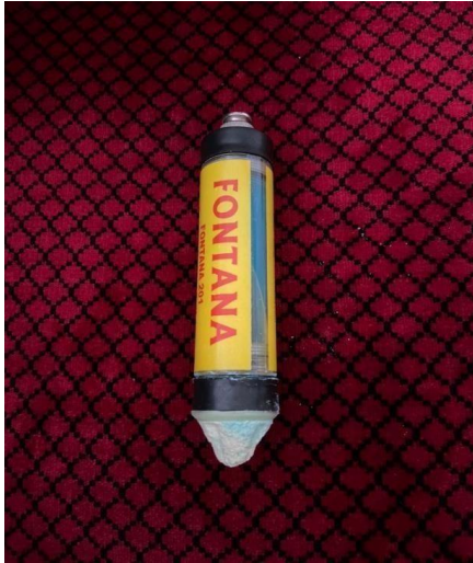
Figure 2: CuSO 4 Reference Electrode
