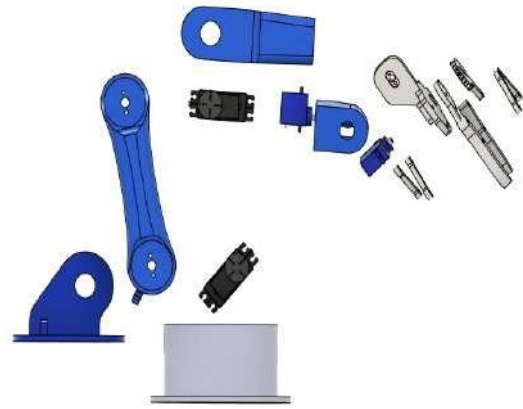
Fig 3- Exploded 3D view of the robotic arm
