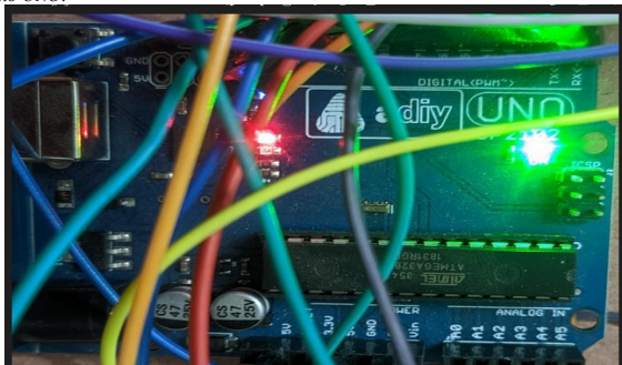
Image 1.1 Arduino UNO used for FRICAS
