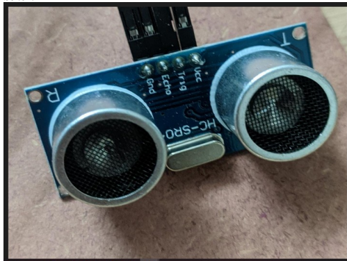
Image 1.5 Ultrasonic Module used in FRICAS
