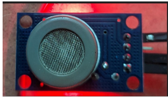
Image 1.2 Fume/Gas sensor used in FRICAS
