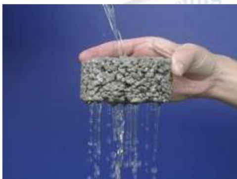
Fig.No.3 Free Draining of porous concrete.
