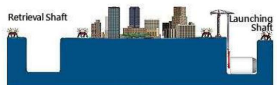
2. Assemble the TBM at the launching shaft
