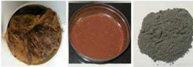
Fig.1. Samples of (b) lateritic soil, (a) coir fiber and (c) fly ash
