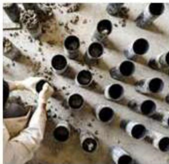
Fig.3. Sample preparation for compaction test
