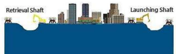
1. Excavate launching shaft and retrieval shaft
