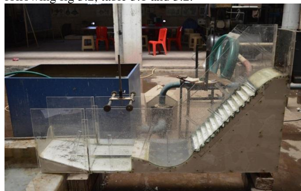
Fig.3.1 Working Model of stepped spillway
