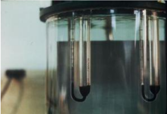
Figure 19. (Viscous flow of modified bitumen)
