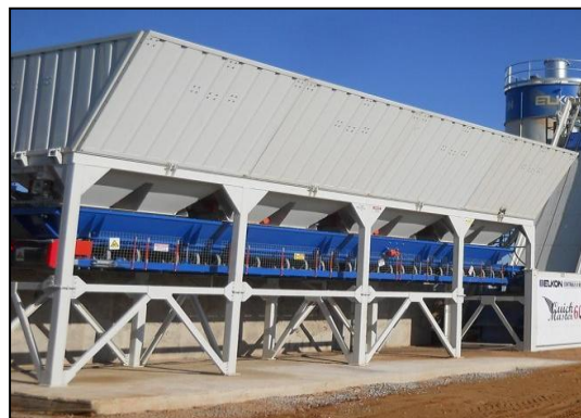
Fig. no. 5.2 Aggregate storage bins
