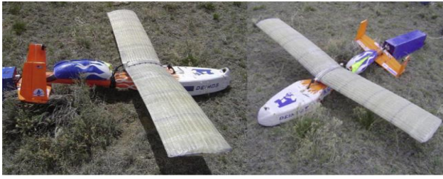
Fig. 5: Big Blue UAV designed at University of Kentucky [11]
