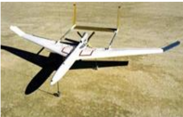
Fig. 2 : Mini-Sniffer -III UAV developed by NASA
