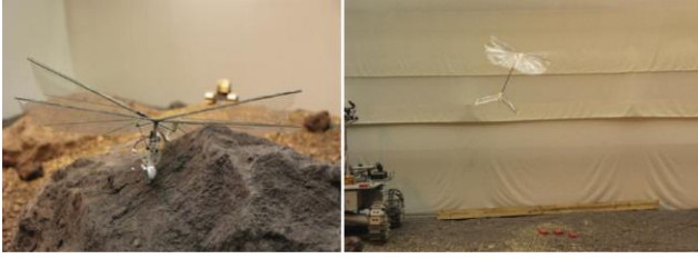
Fig.9: DelFly II from Delft University for use in Earth's atmosphere
