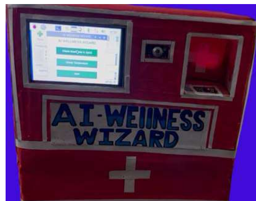
Figure 9. Hardware prototype of AI Wellness Wizard with all sensors and Raspberry Pi Display.
